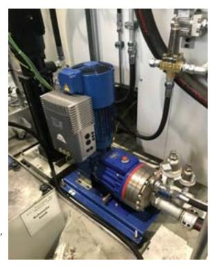
Although it is generally considered adequate to keep the pressure constant and vary the flow according to the tool orifice size, on some occasions (tools with smaller coolant orifices) it is necessary to increase the pressure in order to optimise the cooling capacity.
